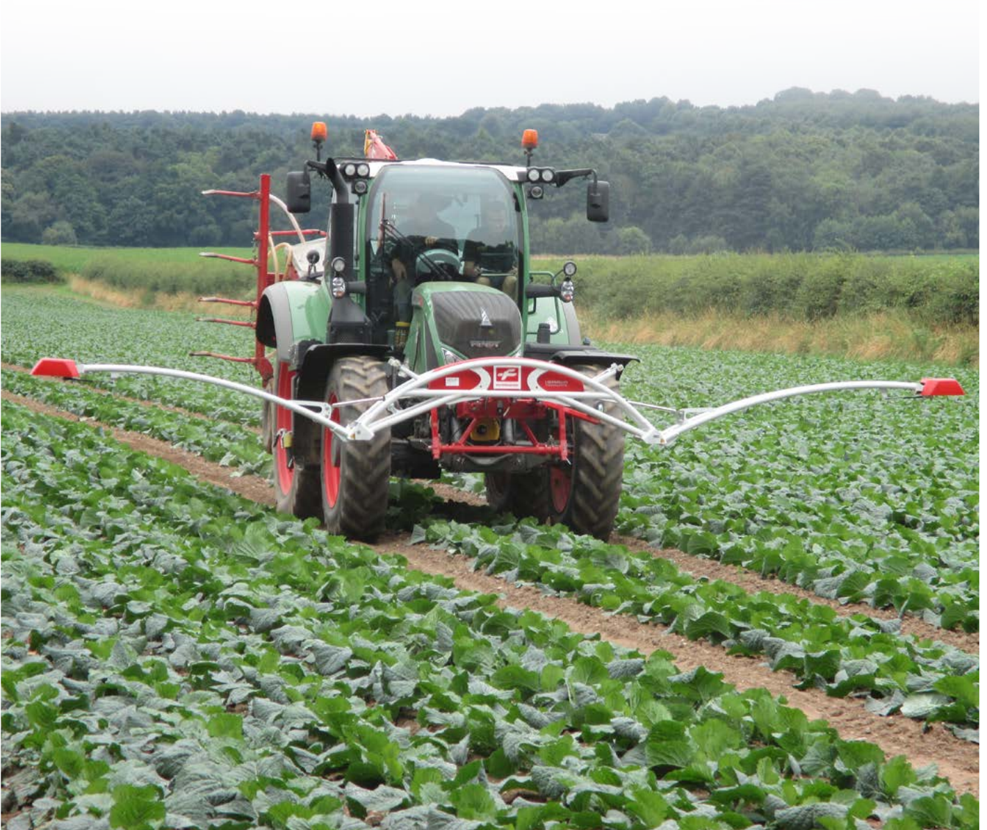
Tractor-mounted Fritzmeier ISARIA crop sensor assessing nitrogen requirements of Savoy cabbage
