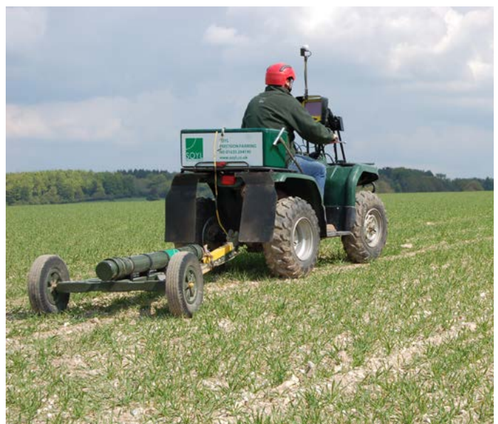
Figure 10. Soil electromagnetic induction (EMI) scanner
